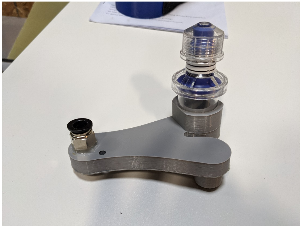
Figure 15 Fully assembled Y-vent in PEEP configuration
